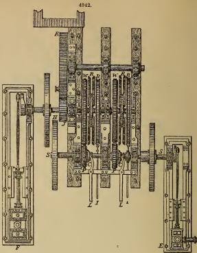
extends beyond the reels, and if the wheel H is moved into gear with the pinion J of the pumpwheel, K may set that in motion. The pumping engine F is commonly used for this purpose, but in case of necessity its work may be done by the hoisting engine E. Lifting may also be performed by the pumping engine, if the wheel H is put in gear with the pinion J. Thus, if desired, either engine may serve as a substitute for the other.
